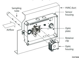
Fig. 25 - Sensor Cleaning Diagram
